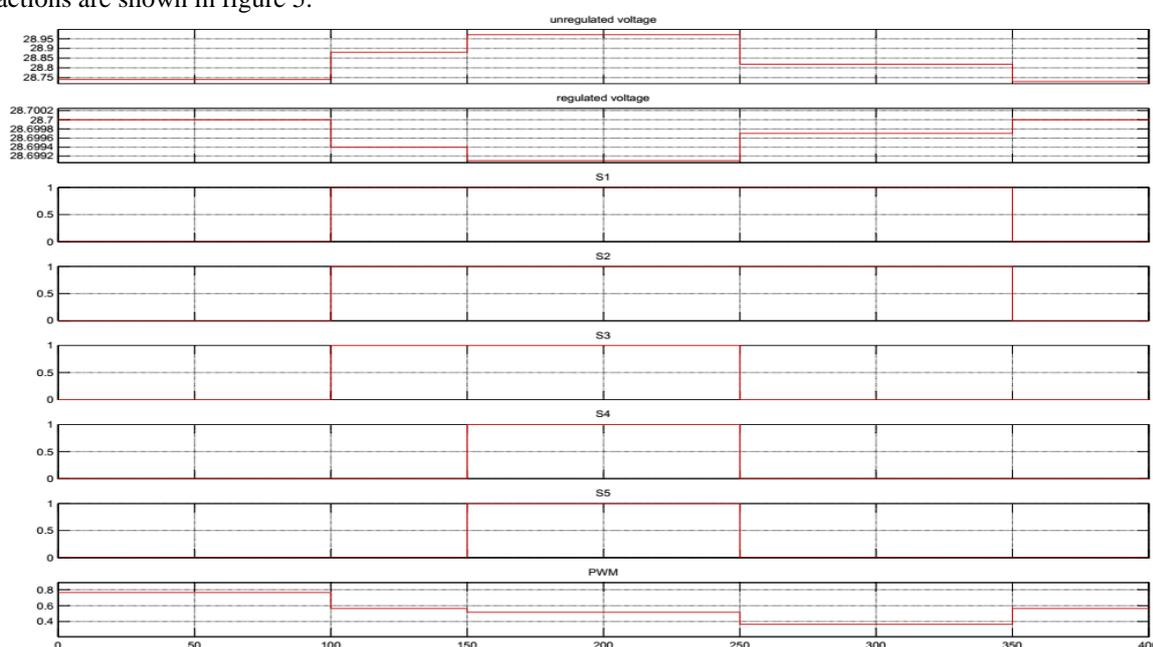
**Figure 5** Bus voltage response and corresponding control actions
