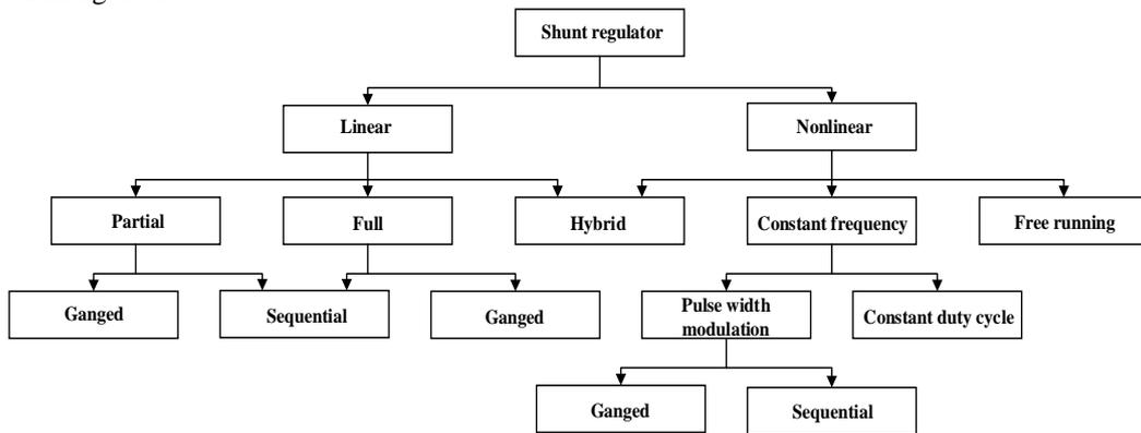
Figure 1 Solar arrays shunt regulators methodologies
