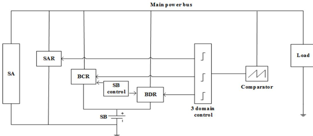
Figure 2 Ordinary control components in fully regulated voltage power bus
