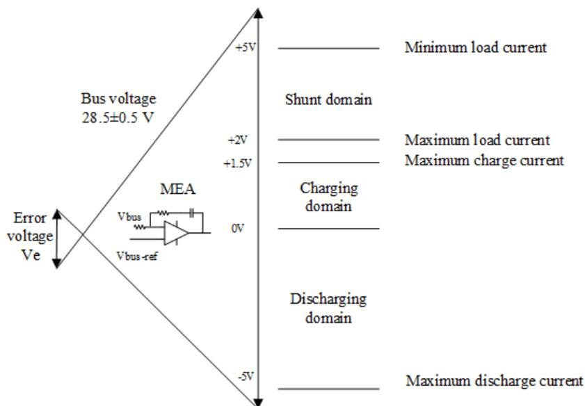
Figure 3 Operating domains of PSS versus bus error voltage
