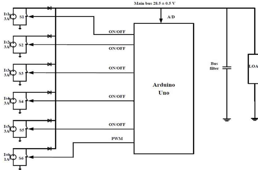
Figure 4 Proposed shunt regulator architecture
